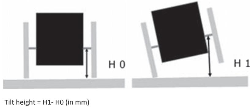
Fig. 2. Measurement of the height of the tilt in the tilt test.
