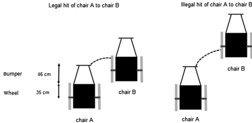
Fig. 3. Example of a legal and an illegal hit based on the position of two wheelchairs (drawing not to scale).
