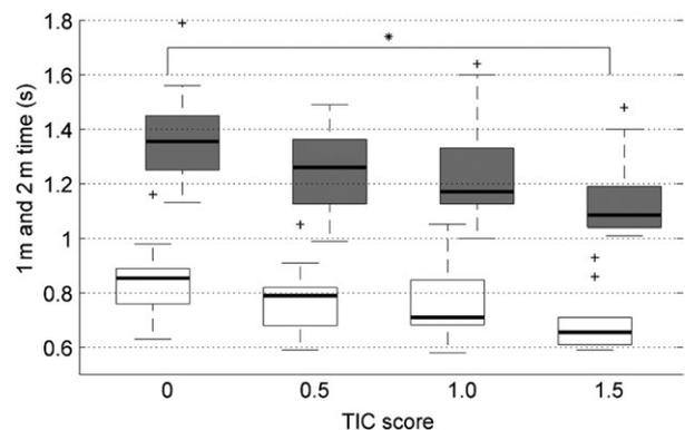
Fig. 7. Boxplot of the time to push 1 m and 2 m in the acceleration test per TIC score. Lower (white) box plots represent the time to push 1 m. Upper (gray) box plots represent the time to push 2 m. Middle line = median, Lower margin = lower quartile, Upper margin = upper quartile, Whiskers = range, + = extreme value, \* = significant difference between the TIC scores for both time to push 1 m and 2 m.
